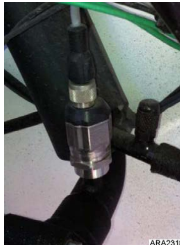
Suction Transducer Installed
