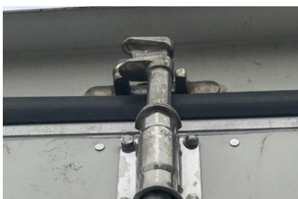
Figure 5.1.22 Lock rod in secure position top.
