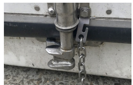
Figure 5.1.23 Lock rod in secure position bottom.
