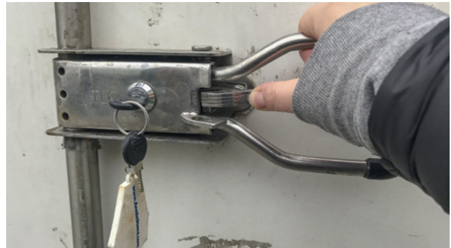
Figure 5.1.16 Press in the lock closing device.
