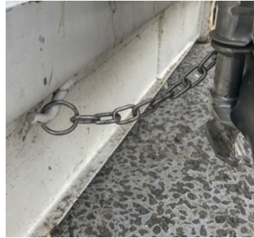
Figure 5.1.26 The chain is secured to the hook on both sides of the container.
