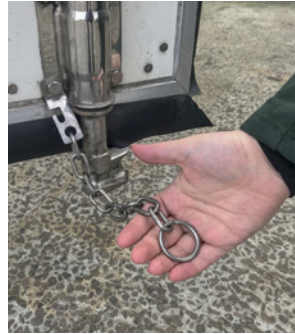
Figure 5.1.25 The safety chain is placed at the bottom of the doors
