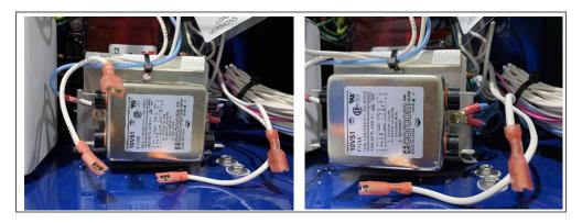
3. Remove the remaining mounting bolt on the left side (line input) and pull from the system control box.
