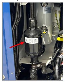
Figure 7.12 Filter Drier
