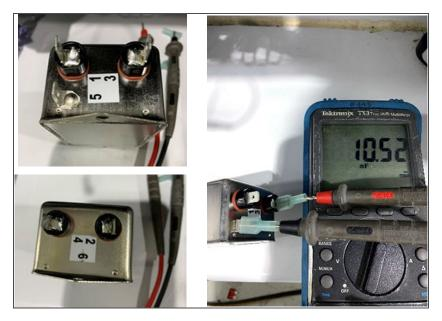
6. Final check on the power filter is to verify the discharge resistor on the power filter output. Check resistance between pins 2 and 4 on the load side of the power filter for  $330k'\Omega$  +/- 10%.
