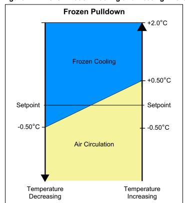
Figure 4.4 Frozen Mode - Cooling and Heating Chart
