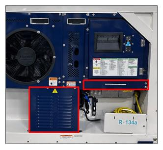
3. Open the VFD service cover to gain access to the fan assembly.
