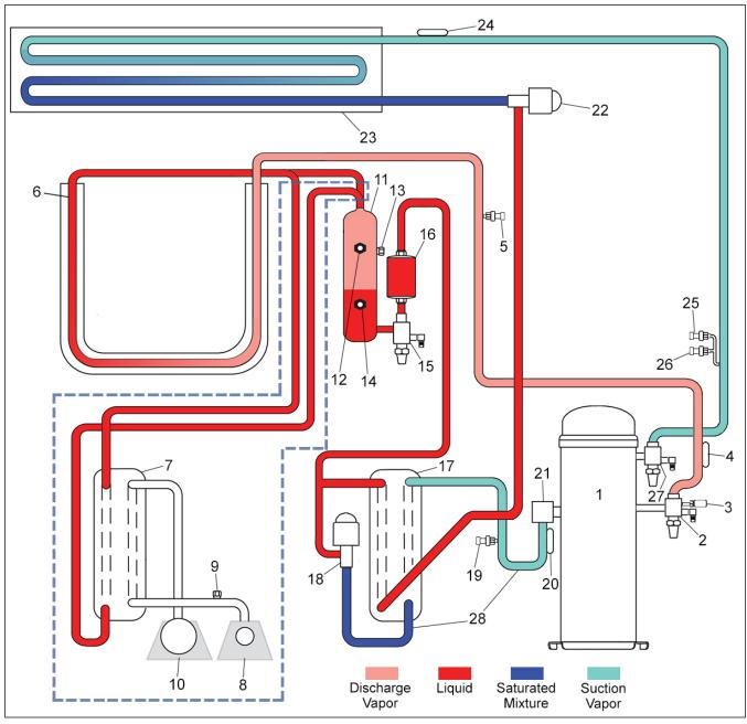
Note: Objects outlined by dashed lines (- - -) indicate an optional water cooled condenser installed.
