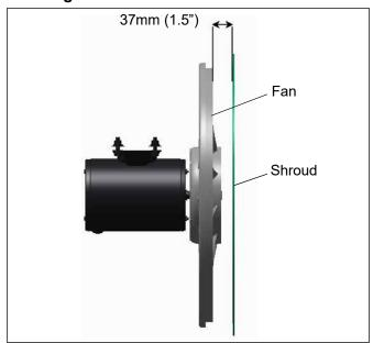
Figure 7.11 Condenser Fan Position
