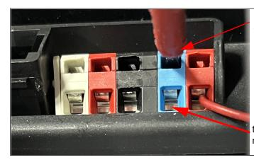
lift screwdriver to open terminal jaws
