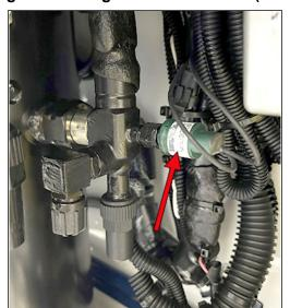
Figure 3.23 High Pressure Switch (HPS)
