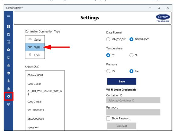
2. Choose the container unit to connect from the Select SSID box. After selecting, the ID is filled into the Container ID box on the right. Type in the password and click Connect. See **Section 4.6.2.1** for container ID and password information.
