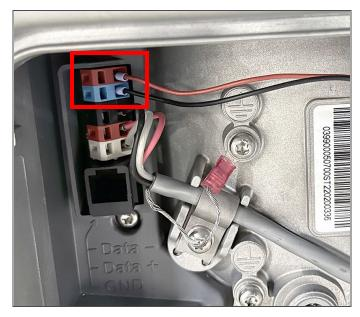
This is done by inserting a small flathead screwdriver in the terminal hole above the wire to be removed, followed by a gentle lifting the screwdriver until the terminal jaws open and the wire is free to be pulled out.
