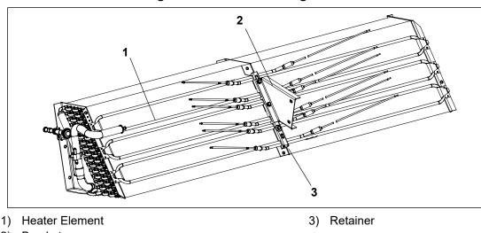
Figure 7.13 Heater Arrangement
