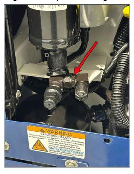
Figure 3.19 Liquid Line / King Valve
