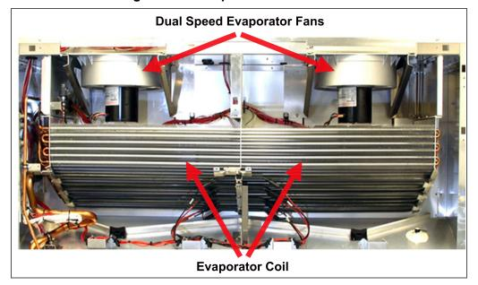
Figure 3.14 Evaporator Coil and Fans
