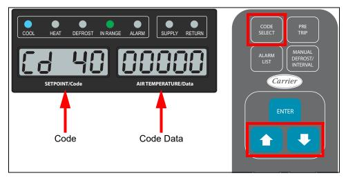
2. Press the ENTER key to navigate into the menu of a selected code. Pressing ENTER will display the present selected value for 5 seconds, or until the user selects a different value. If additional time is required, press ENTER to extend the display time to 30 seconds.
