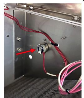
Figure 3.16 Heat Termination Thermostat (HTT)
