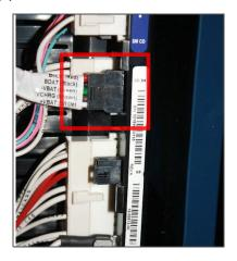
4. Using a Driver Bit, Carrier Transicold part number 07-00418-00, loosen the left hand screw on the battery pack cover then remove the second screw on the outer edge of the battery pack cover.
