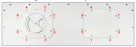
Figure 7.14 Access Panel Torque Pattern
