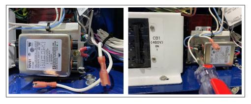
8. Connect wires to the power filter using the hot stamping on the wire harness and pin marking on the power filter.
