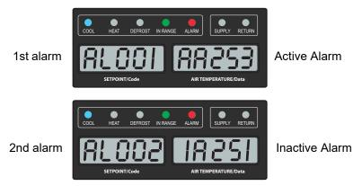
3. "END" is displayed to indicate the end of the alarm list if any alarms are active.
