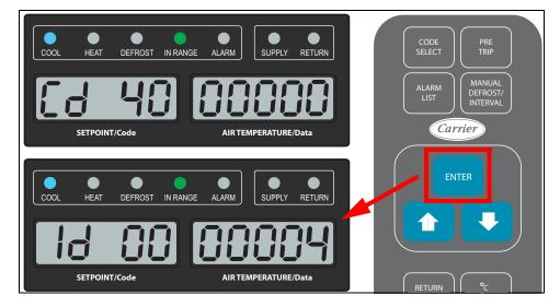
Press the CODE SELECT key while in a selection menu to cancel the current selection and go back up to the higher selection menu. If no key is pressed for 5 seconds, the display reverts to a normal display and the current selection menu is cancelled. Any previously committed changes are retained.
