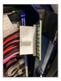
3. Locate the proper wires to be ohmed by referring to the system schematic.
